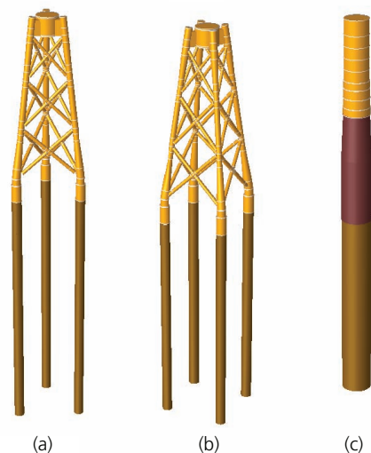
Figure 7. Geometry diagrams for the substructures of offshore WTGs: (a) three-leg jacket type; (b) four-leg jacket type; (c) monopile type
